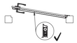
2. If you install the profile on the glass door without frame place activating kit fitting on the glass wall on the closing side of glass door.
